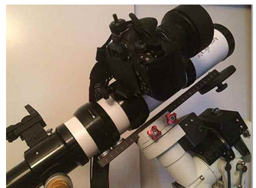
Side view of piggyback adapter washer kludge to allow 2nd clam shell and v-rail clearance (Source: Palmia Observatory)
