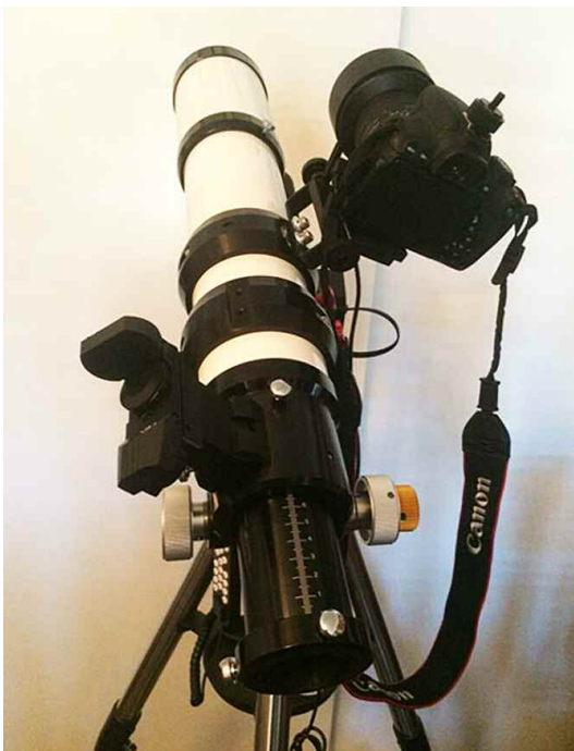
Added piggyback adapter for tracking wide-angle, long exposure images. (Source: Palmia Observatory)
