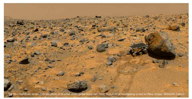
Pathfinder had two parts: a lander that stayed in one place, and a wheeled rover that could move around. The Pathfinder lander had special instruments to study Martian weather. These instruments measured air temperature, pressure and winds. The measurements helped us better understand the climate of Mars.
