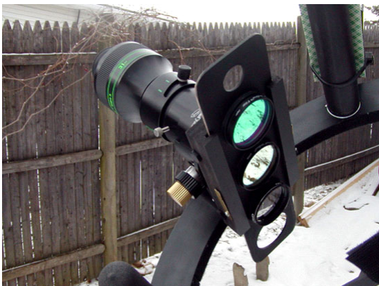
A filter slide provides safe and easy access to your filters. Photo used with permission. www.Astrocrumb.com
