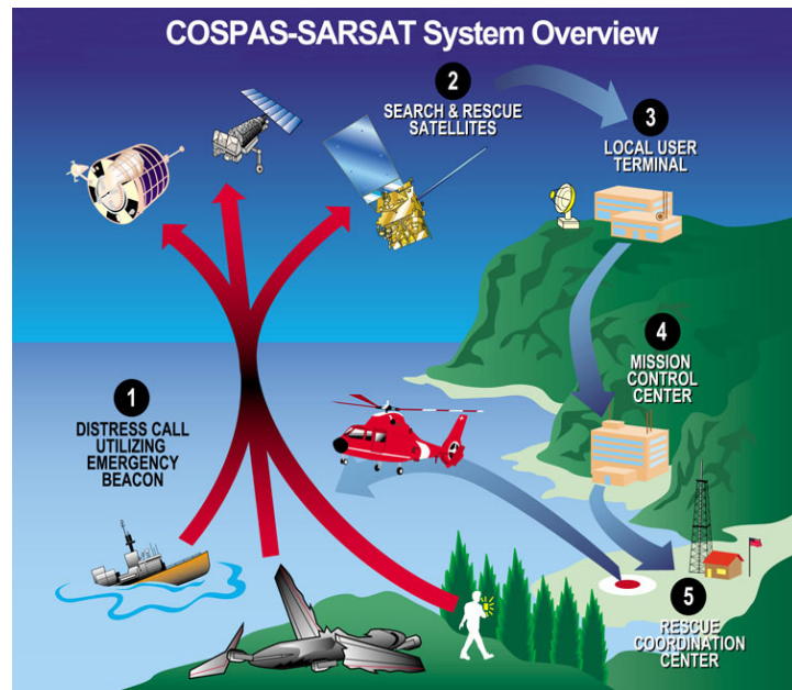
NOAA's polar-orbiting and geostationary satellites, along with Russia's Cospas spacecraft, are part of the sophisticated, international Search and Rescue Satellite-Aided Tracking System.
