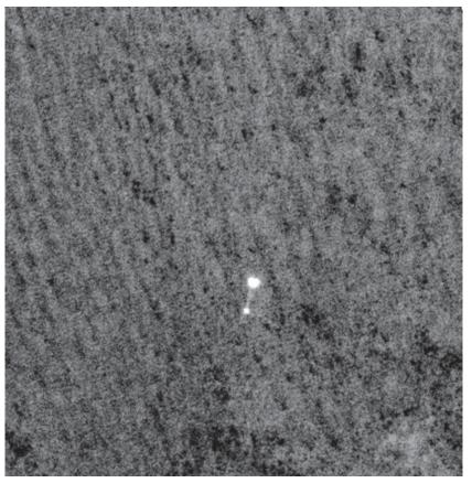
NASA's Phoenix Mars Lander can be seen parachuting down to Mars, in this image captured by the High Resolution Imaging Science Experiment (HiRISE) camera on NASA's Mars Reconnaissance Orbiter. This is the first time that a spacecraft has imaged the final descent of another spacecraft onto a planetary body. (NASA/JPL-Caltech/University of Arizona)
